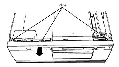
2. To lift the subassembly from the front of the computer, place your thumbs under the diskette drive and grasp the top edge of the computer with the rest of your fingers, as shown in the following illustration. (If you have a diskette drive installed in the lower horizontal drive bay, place your thumbs underneath that drive instead.) Then lift up the subassembly with your thumbs.
